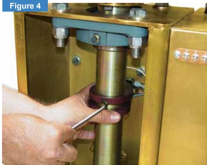
Gate travel is adjusted by loosening the limit Cams and adjusting them until proper gate travel has been achieved.
